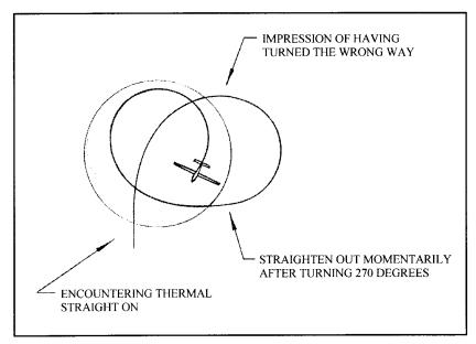
Don't make the mistake of tightening the turn when you are in the sink in an effort to expedite the process of getting back into the lift, if you hold the turn on a bit too long it may have the effect of centering in the sink. Simply maintain the same angle of bank till it's time to straighten out.
